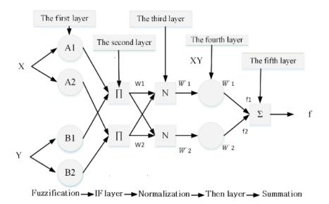
Figure 2. The structure of a neuro-fuzzy system designed in five layers
